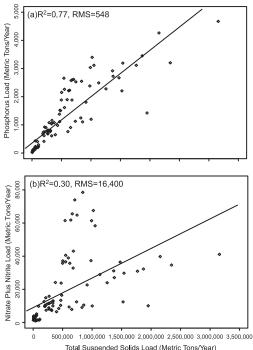
Figure 6.—Comparison of estimated annual loads for 10 years (2000–2010) at nine stations in Indiana for a) total phosphorus and total suspended solids and b) nitrate plus nitrite as nitrogen and total suspended solids, with  $R^2$  and root-mean-square error (RMS). Line represents the regression for each graph.
