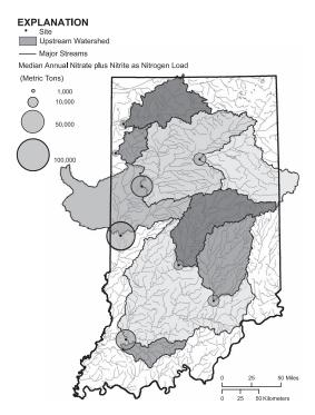
Figure 3.—Median annual loads of nitrate plus nitrite as nitrogen in metric tons per year in Indiana watersheds for the period 2000–2010. Size of circle is proportional to the load.
