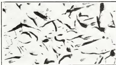
Fig. 1. Gray cast iron. Graphite flakes in matrix of ferrite.  $\times 100$ . (Reduced one-third.)
