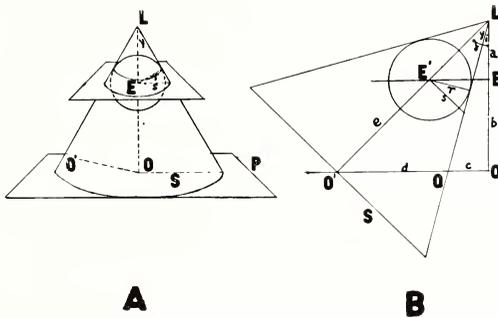
Fig. 8A and B. The projection of spherical sound waves upon a plane surface.
