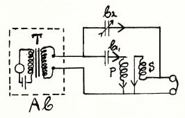
Fig. 1. Diagram showing connections for the apparatus used in the measurement of the amplification constant of an audio transformer.
