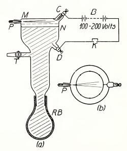
Fig. 1. Apparatus used for demonstrating Alpha-ray tracks. (a), vertical section; (b), cross section at the top.
