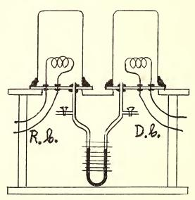
Fig. 1. Drawing showing the differential thermometer. The heat developed in the coil in the left hand beaker by the radio frequency current is balanced by the heat developed in the coil in the right hand beaker by the direct current. The equality of the height of the water in the U-tube indicates when equilibrium is established.
