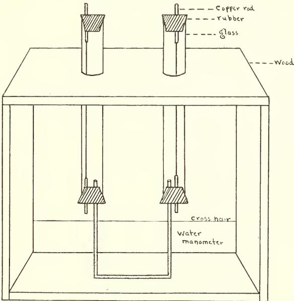
Fig. 1. Device used in the investigation for the calibration of ammeters.
