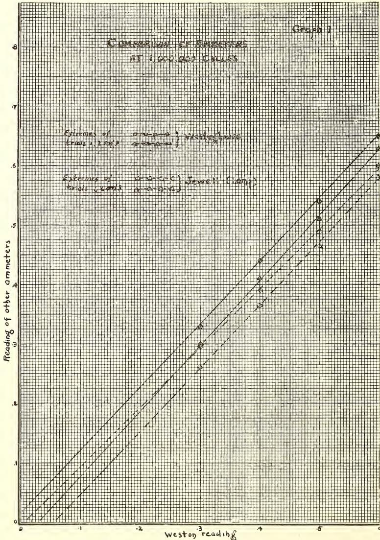
Fig. 3. Comparison of ammeters at 1,000,000 cycles.
