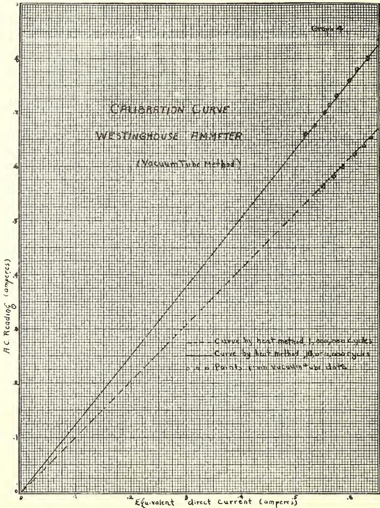
Fig. 12. Comparison of calibration curves as obtained by the heat method at 1,000,000 and 10,000,000 cycles, respectively.
