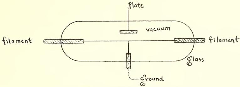
Fig. 8. Construction of tube used in experiments.
