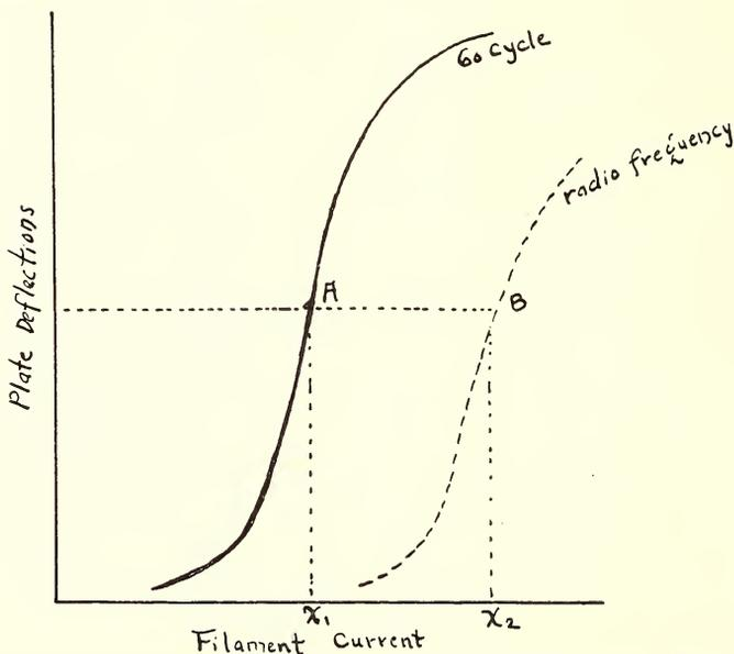
Fig. 10. By comparing the two characteristic curves obtained, the true value of the radio frequency current through the filament is determined.
