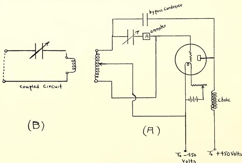
Fig. 2. The oscillator used for production of current is shown in A. The heat apparatus and ammeters to be calibrated were connected in the tuned circuit shown in B.
