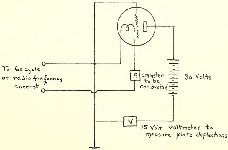
Fig. 9. Arrangement of apparatus and connections used in experiments.
