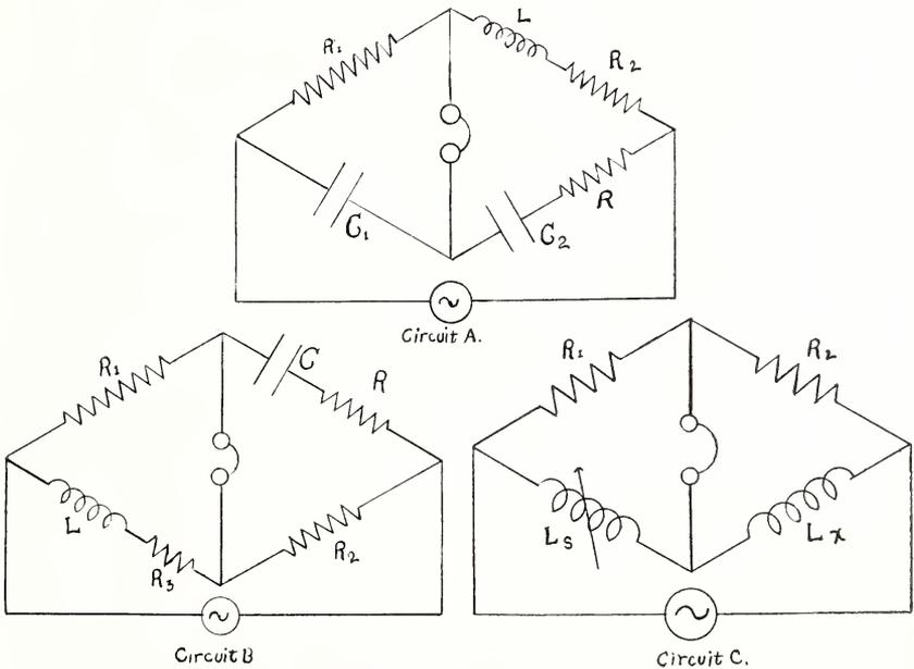
Figure 1. Bridge Circuits.
