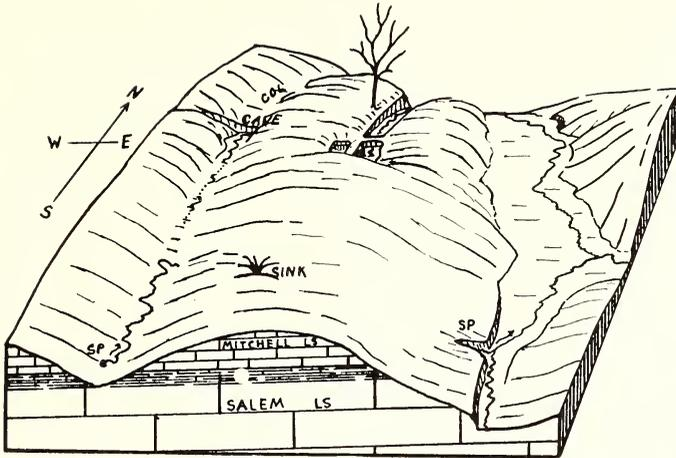
Fig. 3—A generalized block diagram illustrating positional relations of the rock formations and the general topographic condition. The dip of the rock formations and the vertical relief is slightly exaggerated. The finer divisions represented in the upper part of the Salem Limestone are to illustrate the thin layered and shaly phase of that formation.
