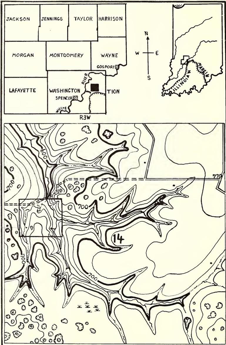
Fig. 1—Topographic map of section 14, township 10 north, range 3 west. The map shows the general topographic condition near the Litten Natural Bridges. The rectangle encloses an area reproduced as figure 2. Contour interval 20 feet.
