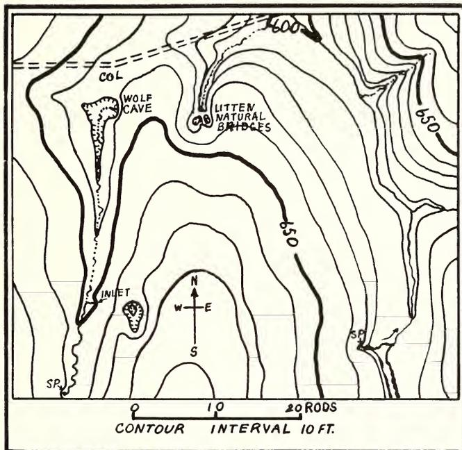
Fig. 2—A reproduction on a larger scale of the rectangle shown in figure 1. The positional relations of the cave, natural bridges, gorge, and abandoned valleys are shown. The figure illustrates successive abandonment of a valley by a surface stream due to subterranean diversion.
