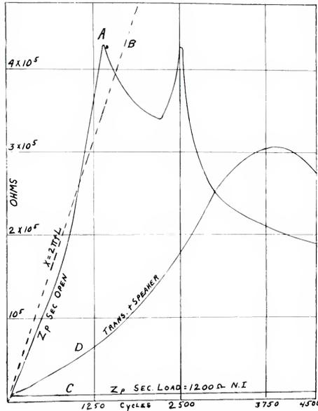
Fig. 1. Impedance curves for output transformer.
