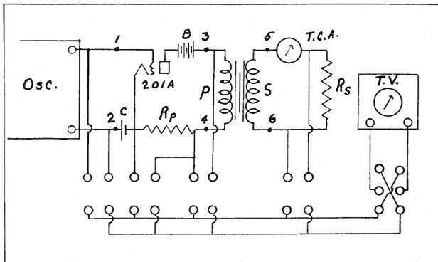
Fig. 3. Measuring circuit for transformer characteristics.
