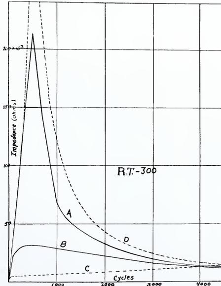
Fig. 6. Impedance curves for interstage transformer.
