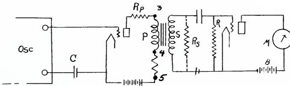
Fig. 5. Transformer impedance measuring circuit.
