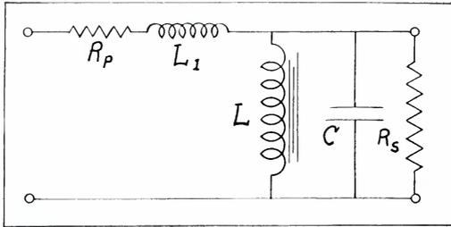
Fig. 2. Equivalent circuit of audio transformer.
