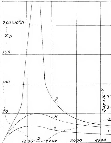
Fig. 7. Series resonance curves.
