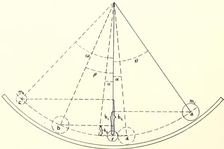
Fig. 2—Diagram used in deriving equation for the coefficient of restitution and the percentage loss of kinetic energy.
