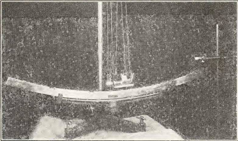
Fig. 1—Apparatus used in testing commercial hammers.
