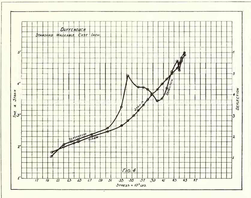
Fig. 4—Stress-Strain and Stress-Deflection curves for machined malleable cast iron.
