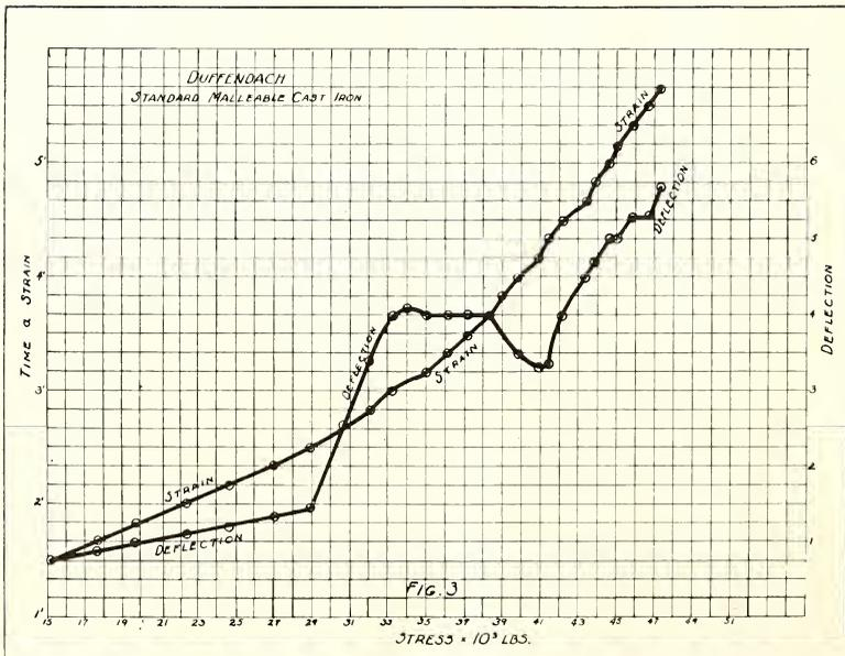
Fig. 3—Stress-Strain and Stress-Deflection curves for malleable cast iron.
