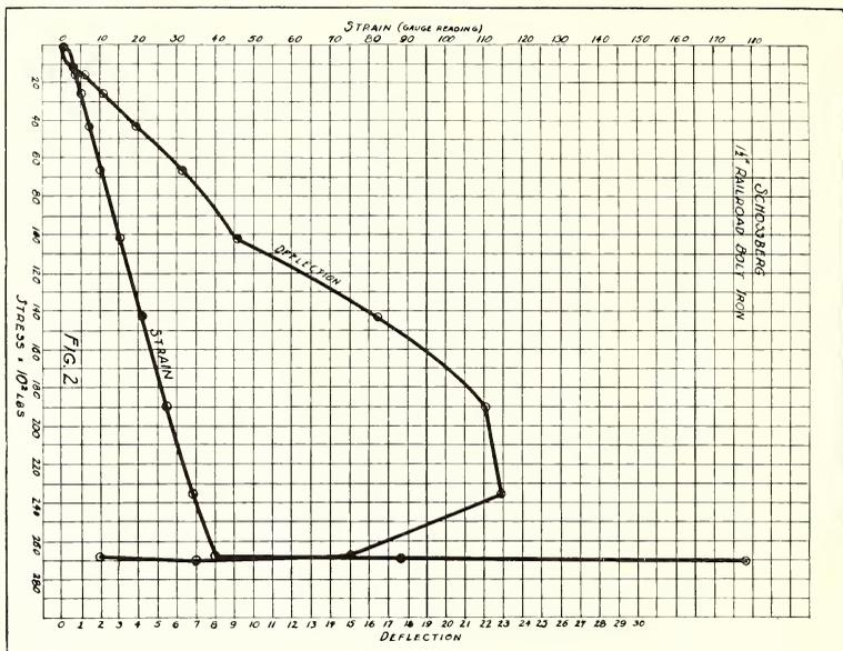
Fig. 2—Stress-Strain and Stress-Deflection curves for wrought iron.
