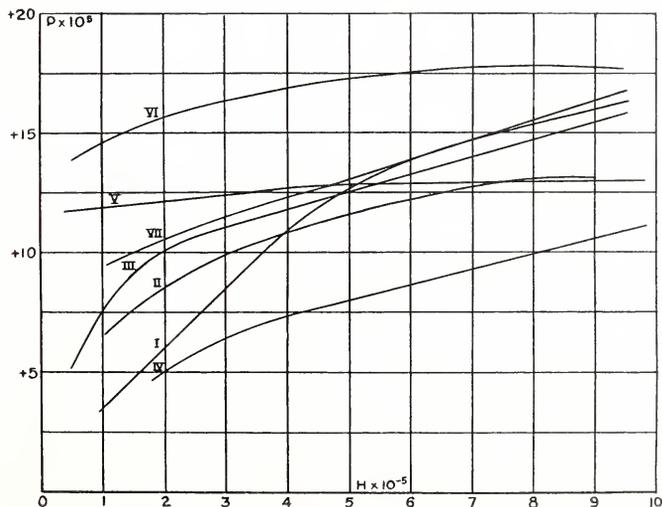
Fig. 3. Ettingshausen Coefficients against Field Intensities.<sup>1</sup>
