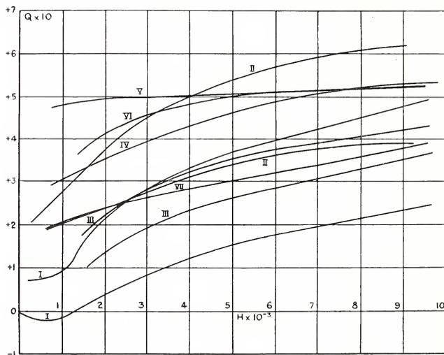
Fig. 4. Nernst Coefficients against Field Intensities.
