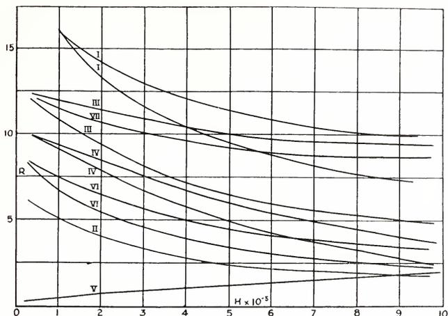
Fig. 2. Hall coefficient against Field Intensities.<sup>1</sup>
