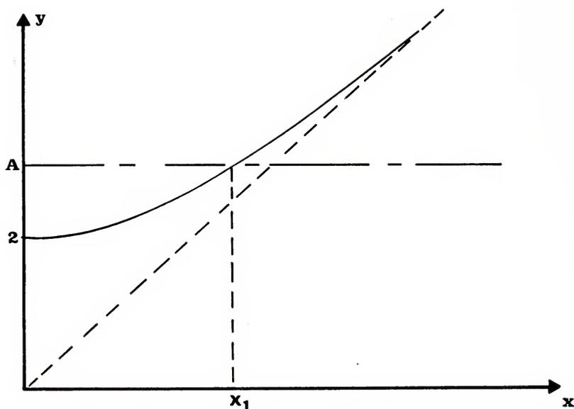
FIGURE 2. Sketch of the graph of  $y=xI_0(x)/I_1(x)$  for  $x > 0$ , from which it is clear that the equation  $y=A$  has one and only one real solution  $x_1$  (say) for every constant  $A > 2$ .
