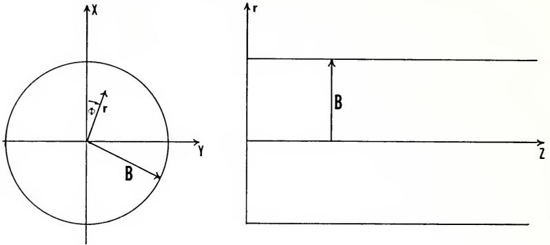
FIGURE 1. From left to right, cross- and longitudinal sections of the domain  $V$ :  $0 \leq r < B, z < \infty$ . The wall impedance boundary conditions are applied at  $r=B$ .
