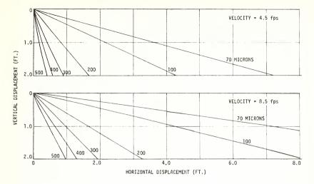
FIGURE 3. THEORETICAL TRAJECTORIES OF SPHERICAL PARTICLES IN A HORIZONTAL AIR STREAM
