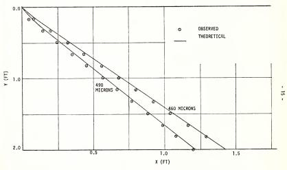
FIGURE 6. THEORETICAL AND OBSERVED TRAJECTORIES FOR A VELOCITY OF 10 FT./SEC.
