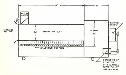
FIGURE 4. A SCHEMATIC DRAWING OF THE SEPARATOR
