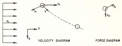
Figure 1. Velocity and Force Diagrams for a Particle in a Horizontal Air Stream.
