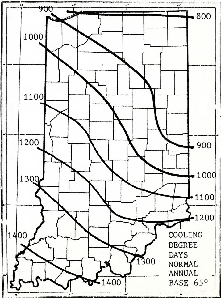
FIGURE 2. Normal annual cooling degree days calculated from daily mean temperatures above 65°F.
