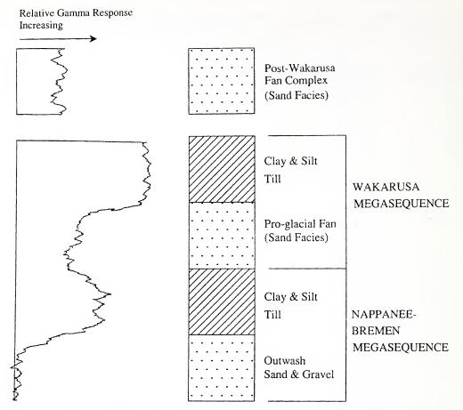
Figure 5.—Idealized gamma Log and Stratigraphic Section, Earthmover's Site, Elkhart, Indiana.
