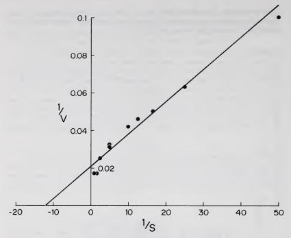
FIGURE 3. Lineweaver-Burke plot of relation between ferricyanide concentration and the rate of ferricyanide reduction by Ascites cells.
