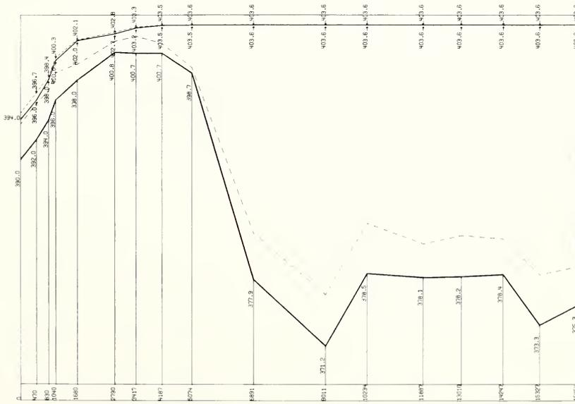
FIGURE 9. Water profile along the Chutes for a discharge of 7550. cfs without the wing dam.
