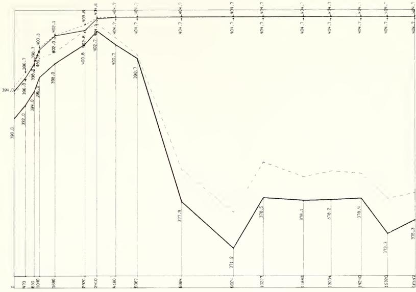
FIGURE 8. Water profile along the Chutes for a discharge of 7550. cfs when the wing dam is present.
