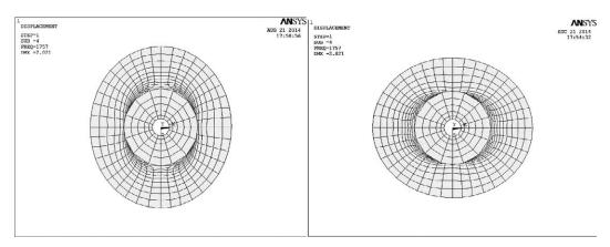
Figure 12.—Two FEA frames of opposite extreme displacement for the (2,0) mode.
