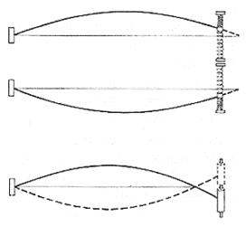
Figure 4.—Relaxing boundary conditions at one end of a vibrating string under tension (from Weinreich<sup>3</sup>).
