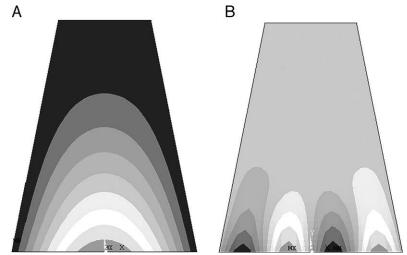
Figure 7.—Flat trapezoidal plate. A. Mode (0,0). B. Mode (3,0).
