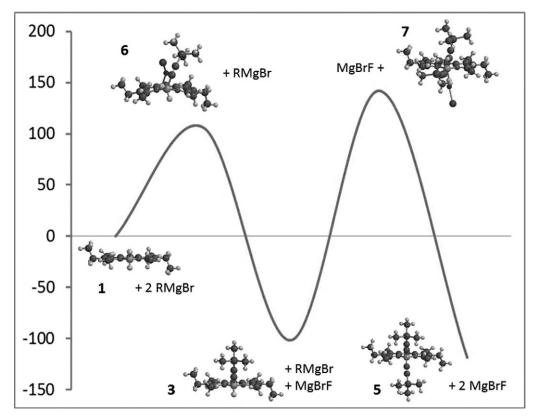
Figure 4.—Energy profile for the substitution of fluorine on F-BODIPY with magnesium bromide ethynyl anion. R = trimethylsilylacetylide anion.
