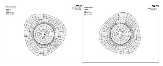
Figure 14.—Two FEA frames of opposite extreme displacement for the (3,1) mode. The nodal line lies approximately between the fourth and the fifth circumferential grid line.
