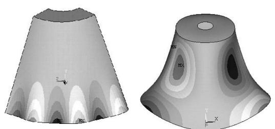
Figure 9.—Conical plate section with crown. Mode (5,0).
