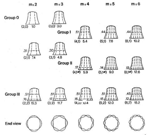
Figure 2.—Systematic grouping of modes of vibration in a hand-bell (from Rossing & Perrin<sup>2</sup>).
