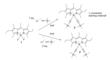
Scheme 2.—Synthesis of E-BODIPY using ethynyl anion generated with n-butyllithium.
