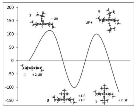
Figure 2.—Energy profile for the substitution of fluorine on F-BODIPY with lithium ethynyl anion. R = trimethylsilylacetylide anion.
