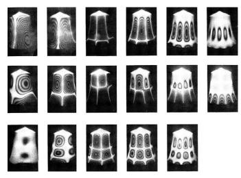
Figure 1.—Vibrational modes of a hand-bell imaged with holographic interferometry (from Rossing, Perrin, Sathoff & Peterson<sup>1</sup>).
