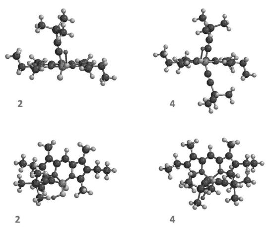
Figure 1.—Transition state models with lithium cation(2 for monosubstitution and 4 for disubstitution).
