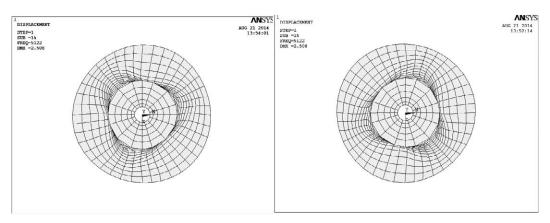
Figure 16.—Two FEA frames of opposite extreme displacement for the (3,1) mode. The nodal line is located between the rim and the first circumferential grid line.
