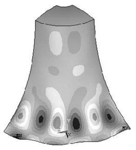
Figure 10.—Bell section with double curvature. Mode (5,1).
