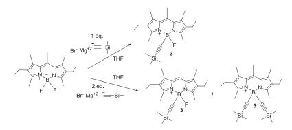
Scheme 3.—Synthesis of E-BODIPY using ethynyl anion generated with a Grignard reagent.
