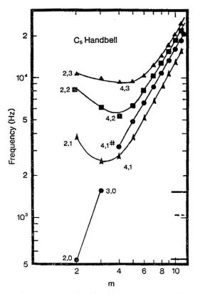
Figure 3.—Relationship of frequency and first mod index of a  $C_5$  Hand-bell (from Rossing, Perrin, Sathoff & Peterson<sup>1</sup>).
