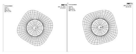
Figure 15.—Two FEA frames of opposite extreme displacement for the (4,1) mode. The nodal line lies approximately between the fourth and the fifth circumferential grid line.
