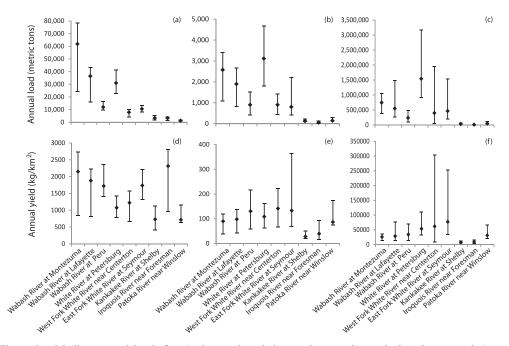
Figure 2.—Median annual loads for a) nitrate plus nitrite as nitrogen, b) total phosphorus, and c) total suspended solids, and annual yields for d) nitrate plus nitrite as nitrogen, e) total phosphorus, and f) total suspended solids. Diamond represents the mean annual load from 2000–2010. Whiskers represent the range of values for annual load (min and max) for each of the nine Indiana watersheds.
