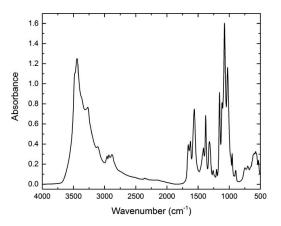
Figure 1.—Representative IR obtained from lobster with a degree of acetylation (DA) of 24.9%.
