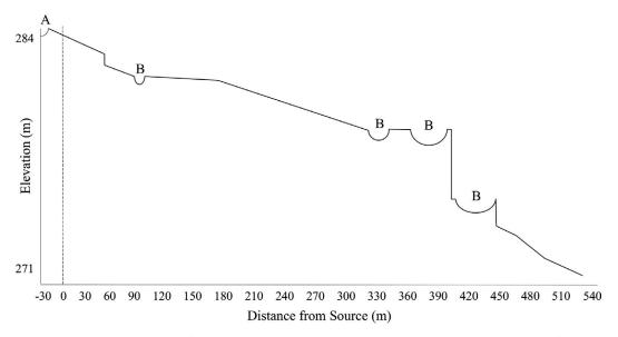
Figure 1.—Elevation change from geothermal discharge source (dashed line) to lake. The lake-fed pool location (A) at -30 m above the source and settling basins (B) at 90 m, 330 m, 390 m, and 420 m are also shown.
