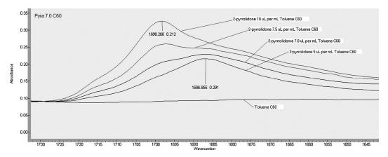
Figure 4.—The spectra of 10.0  $\mu$ L, 7.5  $\mu$ L, 7.0  $\mu$ L, & 5.0  $\mu$ L of 2-pyrrolidone per mL of toluene saturated with C<sub>60</sub> are shown to clarify the carbonyl shift from near 1698 cm<sup>-1</sup> to near 1687 cm<sup>-1</sup>.
