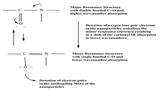
Figure 6.—A resonance structure model suggesting oxygen, lone pair donation to the nanoparticles ( $C_{60}$ ) that shifts stability toward the resonance structure with the single bonded carbonyl and supports a shift of the carbonyl absorption to lower wavenumbers.
