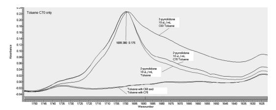
Figure 2.—The spectra of 10  $\mu$ L of 2-pyrrolidone per mL of toluene, per mL of toluene saturated with C<sub>60</sub>, and per mL of toluene saturated with C<sub>70</sub> are shown. In addition, the spectra of toluene saturated with C<sub>60</sub> and toluene saturated with C<sub>70</sub> are included.
