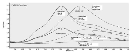
Figure 3.—The spectra of 5 and 2  $\mu$ L of 2-pyrrolidone per mL of toluene, per mL of toluene saturated with C<sub>60</sub>, and per mL of toluene saturated with C<sub>70</sub> are shown. In addition, the spectra of toluene saturated with C<sub>60</sub> and toluene saturated with C<sub>70</sub> are shown.
