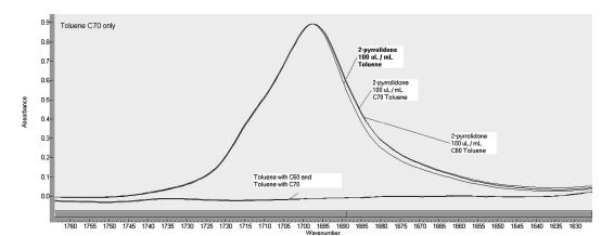
Figure 1.—The spectra of 100  $\mu$ L of 2-pyrrolidone per mL of toluene, per mL of toluene saturated with C<sub>60</sub>, and per mL of toluene saturated with C<sub>70</sub> are shown. In addition, the spectra of toluene saturated with C<sub>60</sub> and toluene saturated with C<sub>70</sub> are included.
